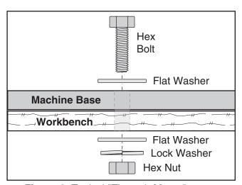
Figure 6. Typical "Through Mount" setup.
